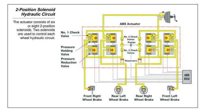
Pressure Holding Valve The pressure holding valve controls (opens and closes) the circuit between the brake master cylinder and the wheel cylinder. The valve is spring loaded to the open position (normally open). When current flows in the coil the valve closes. A spring loaded check valve provides an additional release passage when pressure from the master cylinder drops.
