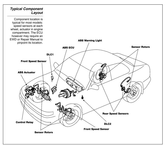
Wheel Speed Sensor A wheel speed sensor is mounted at each wheel and sends a wheel rotation signal to the ABS ECU. The front and rear wheel speed sensors consist of a permanent magnet attached to a soft iron core (yoke) and a wire wound coil. The front wheel speed sensors are mounted to the steering knuckle, and the rear speed sensors are mounted to the rear axle carrier. Serrated rotors are mounted to the drive axle shaft or brake rotor, and rotate as a unit.
