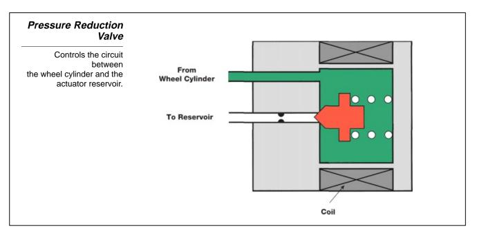
Operation During Normal Braking (ABS Not Activated)
