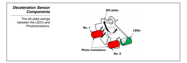
Operation Both LED's are located on one side of the slit plate and both photo transistors are located on the opposite side. The LED's are ON when the ignition switch is in the ON position. When the vehicle's rate of deceleration changes, the slit plate swings in the vehicle's rear-to-front direction. The slits in the slit plate act to expose the light from the LEDs to the phototransistors. This movement of the slit plate switches the phototransistors ON and OFF.
