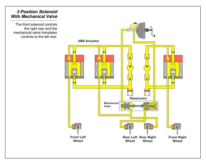
3-Position Solenoids The 3-position solenoid valve actuator comes in three solenoid or four solenoid configurations. The four-solenoid system controls hydraulic pressure to all four wheels. In the 3-solenoid system, each front wheel is controlled independently while the rear wheels are controlled in tandem.
